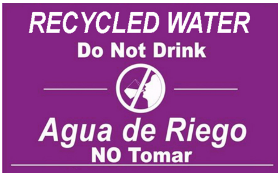
Figure 4-2: Example of Sign on Appurtenances and at Access Points to Parcels Served with Recycled Water
